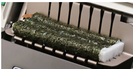
3 pieces of thin size roll can be set on cutting table: 1,650 rolls/hr.
