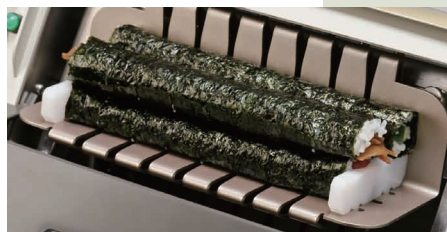
4 pieces of thin size of Norimaki can be cut : 2,200 rolls/hr.
